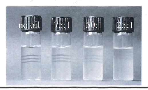
**NOTES.** This kit detects oil by forcing it to form bubbles. Familiarity with results will enable the user to accurately estimate the ratio of oil/petrol. It is recommended that new users test a known sample to use as a reference.
